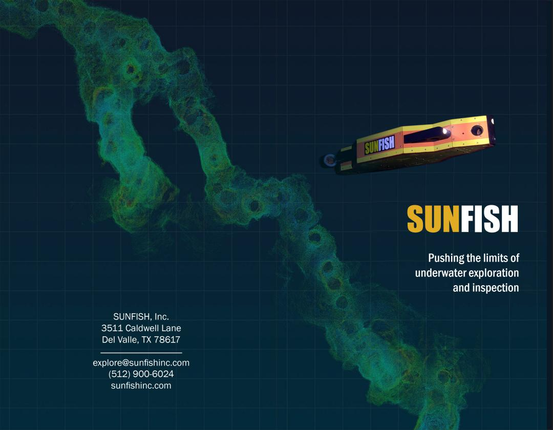
SUNFISH is a person-portable, 6-degree of freedom autonomous underwater vehicle that moves in any direction, assumes any orientation, and independently rotates about any axis. This unique maneuverability allows SUNFISH to sense the environment, acquire data, and build full 3D maps in ways previously unattainable.
